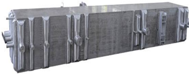
Fig.2 Illustration of a Typical Multi-Stream Brazed Aluminium Plate-Fin Heat Exchanger. [1]
